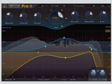
Pro-R's Decay Rate EQ lets you freely scale the decay time across the frequency spectrum
